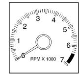
The tachometer displays the engine speed in revolutions per minute (rpm).
